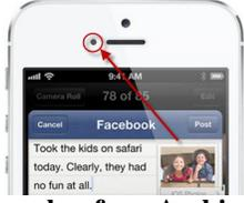
**Fig. 1: The example of an Ambient Light Sensor**
